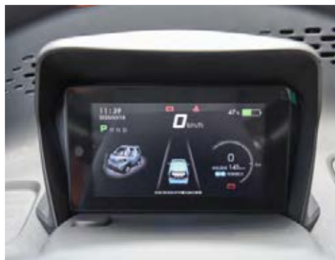
It has a tablet-style central control system
