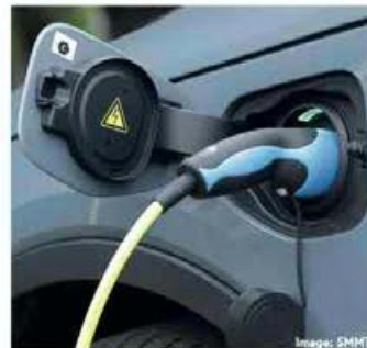
Chargers lock in place when cars lock
