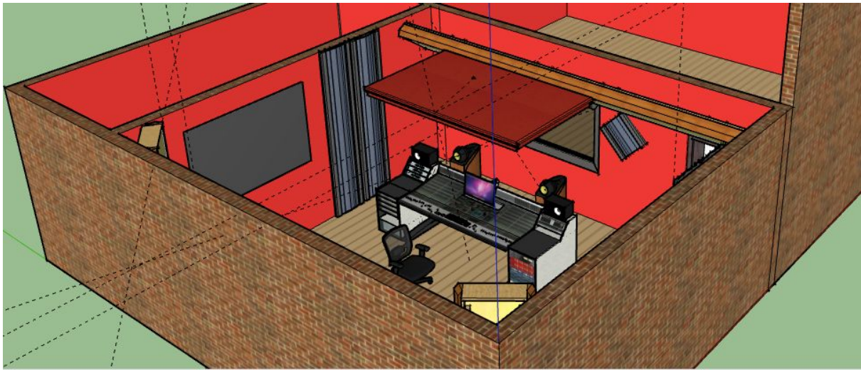
FIGURE 14 - CONTROL ROOM AFTER ACOUSTIC TREATMENT – SIDE VIEW 1
