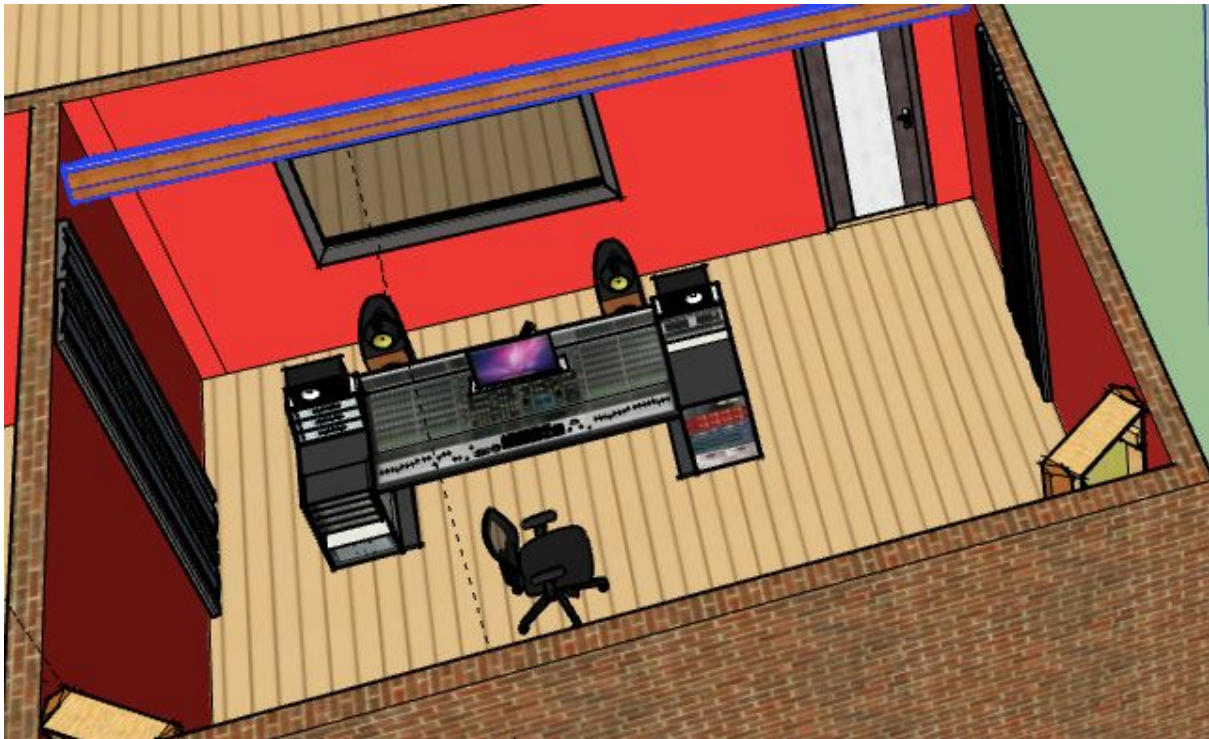
FIGURE 11 – SIDE ABSORPTION TILES
